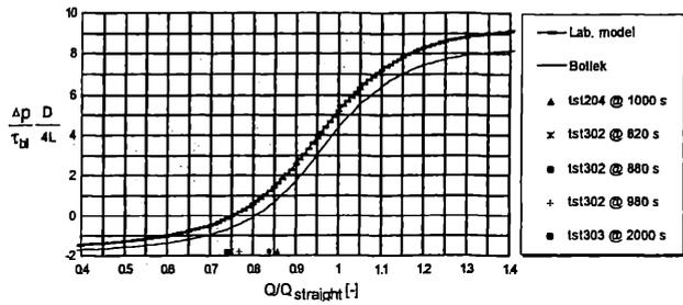
Figure 3a. Mathematical model screw conveyor (geometry model tests:  $S/D = 0.70$  and  $D_r/D = 0.45$ , Botlek Rail Tunnel:  $S/D = 0.63$  and  $D_r/D = 0.22$ ). Dimensionless flow rates in model tests are indicated on the ordinate.
