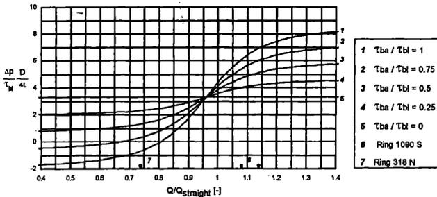
Figure 3b. Mathematical model screw conveyor: Botlek, variation of ratio  $\tau_{ba}/\tau_{bl}$ . Dimensionless flow rates for two situations being analysed are indicated on the ordinate.
