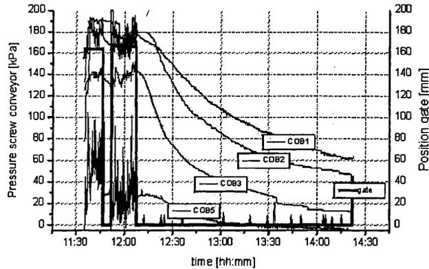
Figure 6. Botlek Rail Tunnel: pressure gauges along the screw conveyor as a function of time: South tube, Ring 1090. For  $t > 12:10$  the excavation is halted and tunneling segments are placed.
