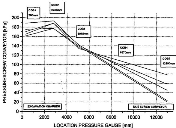
Figure 7. Botlek Rail Tunnel: pressure distribution along screw conveyor during excavation at different time-instances: South tube, Ring 1090.
