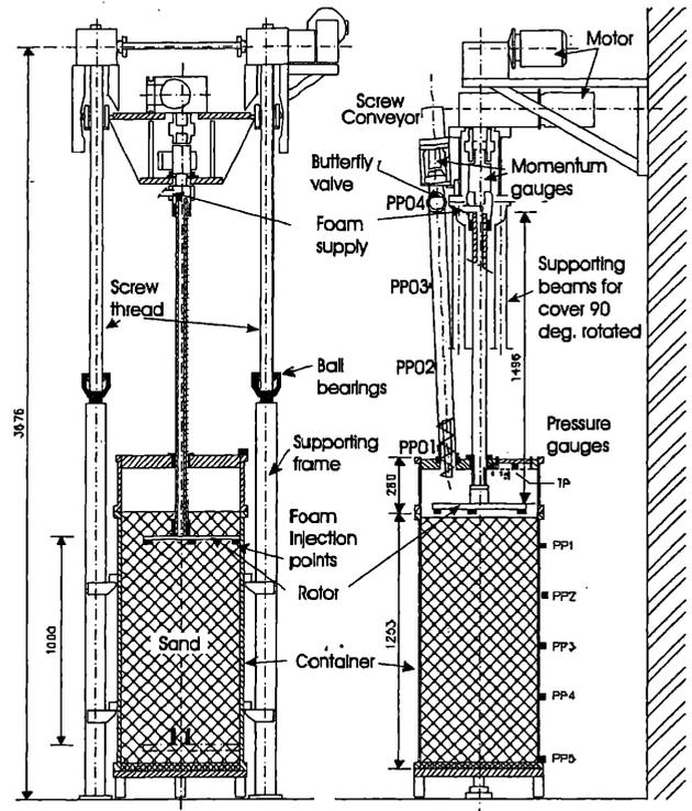
Figure 4. Set-up model test.
