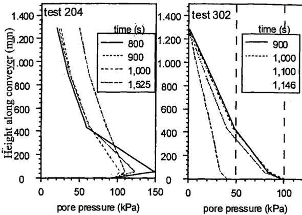
Figure 5. Measured/pressure distribution over model screw conveyor.
