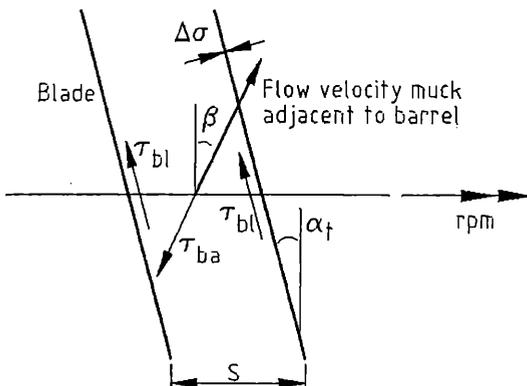
Figure 2. Definition sketch mathematical model screw conveyor, relating geometry, operational conditions and stresses.
