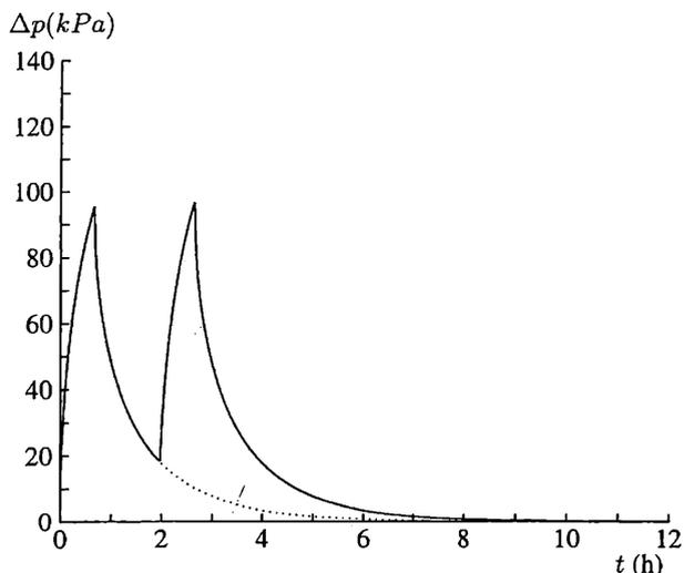
Figure 3. Excess pore pressures generated at the face due to infiltration.
