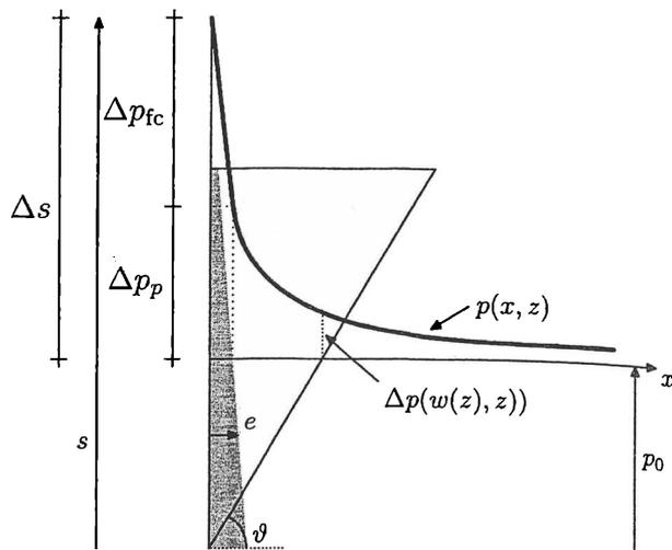
Figure 2. Pressure drop over the slurry infiltration zone and excess pore pressure distribution.
