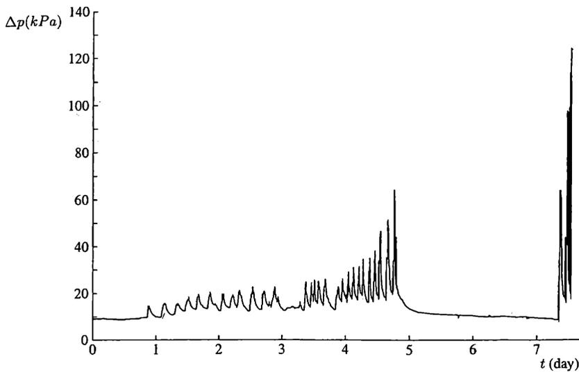
Figure 4. Pore pressure measurements for Botlek Rail Tunnel MQ1 as function of time (BTC/NS-RIB 2000).
