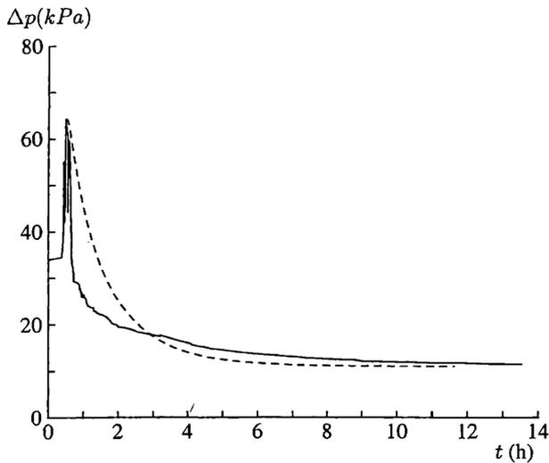
Figure 5. Pore pressure measurements for MQ1, ring 67, compared with (5) for  $x = 4.5\text{m}$ .
