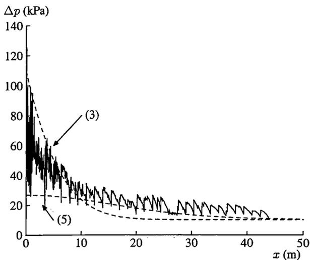
Figure 6. Excess pore pressure profiles according to (3) at  $t = 0.75h$  and (5) at  $t = 1.5h$ , compared with measurements for MQ1.
