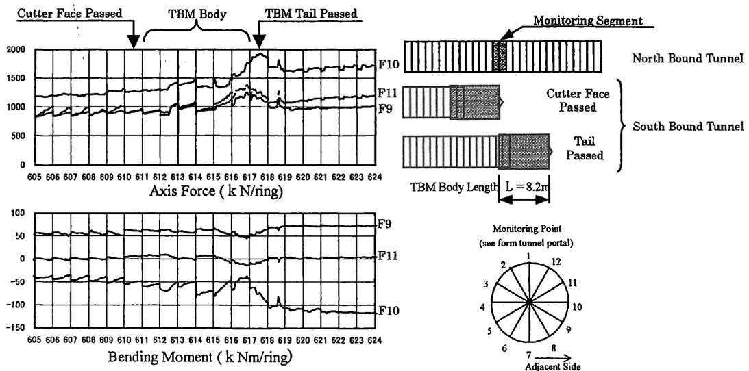
Figure-3 Axis Force, Bending Moment Graph at the Ring of Passing
