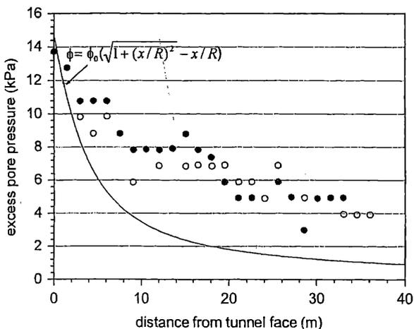
Figure 5: Measured excess pore pressure in front of an EPB shield (• pore pressure gauge 1, o pore pressure gauge 2) and approximation (Botlek Rail Tunnel, MQ4 South). Relatively permeable subsoil (measurement data from Hoefsloot, 2001).
