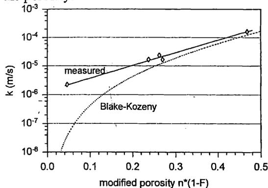
Figure 1. Permeabilities measured in a foam mixture compared with the Blake-Kozeny equation assuming that the foam only reduces the porosity. Figure modified from Kleinjan & Hannink (1999).  $F$  is the volume of air
