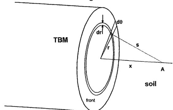
Figure 2. Sketch of tunnel face for flow computation.
