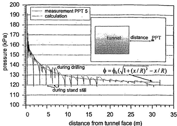
Figure 3: Measured excess pore pressure in front of a slurry shield and approximation (2<sup>nd</sup> Heineoord Tunnel).
