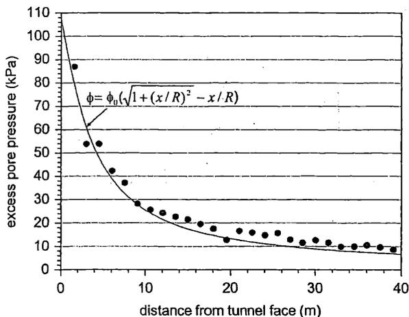
Figure 4: Measured excess pore pressure in front of an EPB shield (•) and approximation (Botlek Rail Tunnel, MQ1 South). Relatively impermeable subsoil (measurement data from Hoefsloot, 2001).
