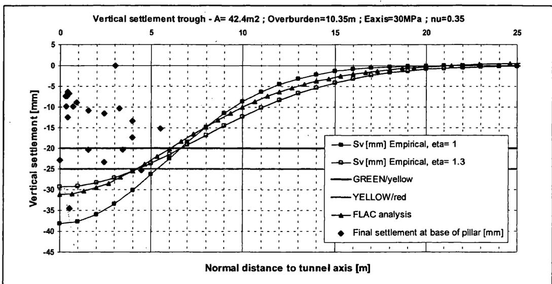
Fig.11 Estimated settlement envelope vs. measured settlements.
