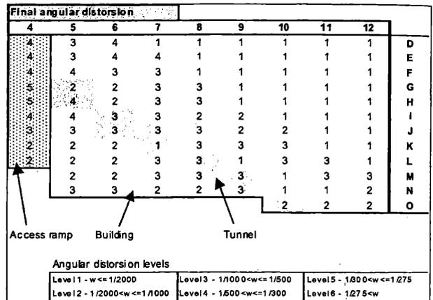
Fig.8 Final angular distortion at the end of excavation of the tunnel.
