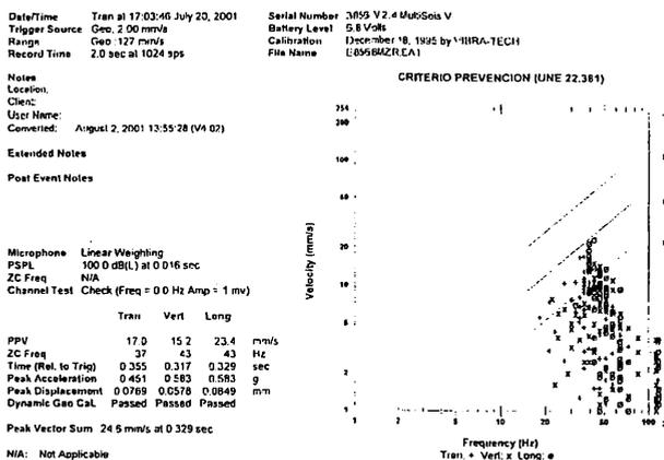
Fig.6 UNE 22-381-93. Damage criteria prevention against vibration induced by blasting.
