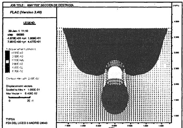
Fig.10 Vertical calculated displacement [m] at the end of tunnel construction.
