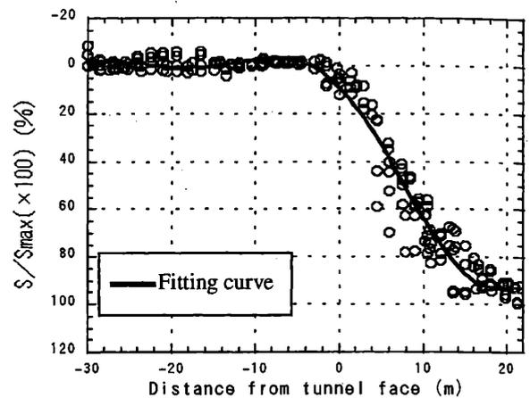
Figure 8 Relationship between surface and sub-surface settlement and tunnel progress
