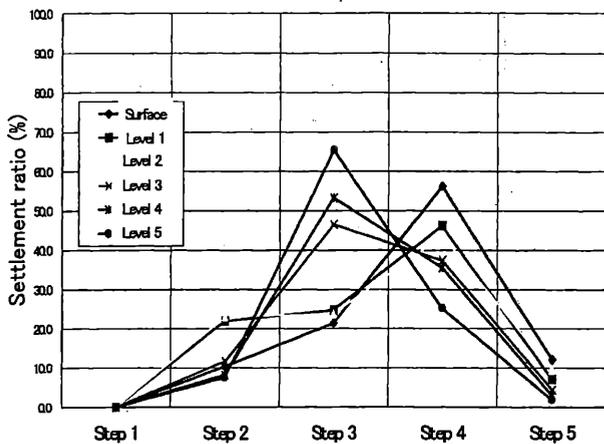
Figure 6 Settlement ratio based on construction process (south bound S3)
