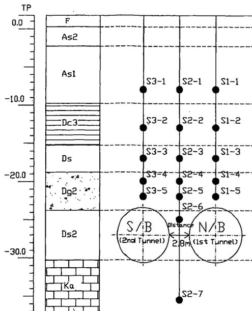
Figure 4 Ground instrumentation (Monitoring site No.2)
