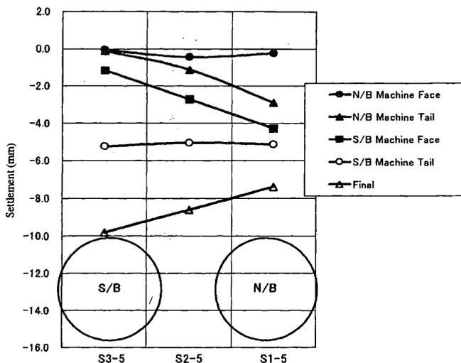
Figure 9 Measurement of ground surface and sub-surface settlements
