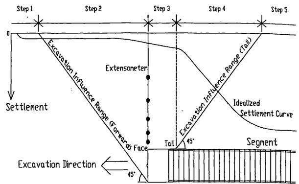
Figure 7 Idealized stages of settlement with respect to time (after Sugiyama, et al.(1999))
