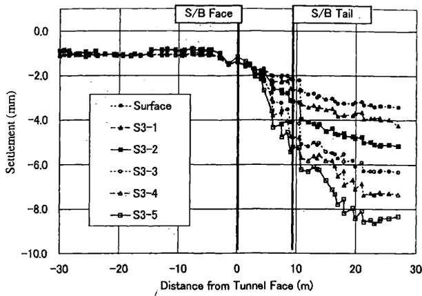
Figure 5 Longitudinal ground surface settlement (Monitoring point B)
