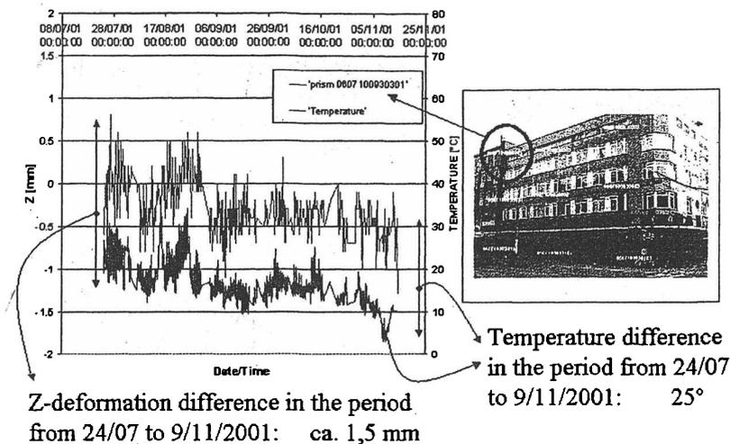
Figure 5: Vertical deformation in relation with the temperature for the first 4 months basic monitoring
