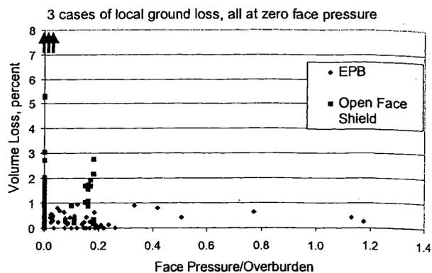
Figure 7. Relationship between face pressure and measured volume loss, EPB and open face shield tunnelling through the Jurong formation, with no Kallang formation soils above the tunnel.
