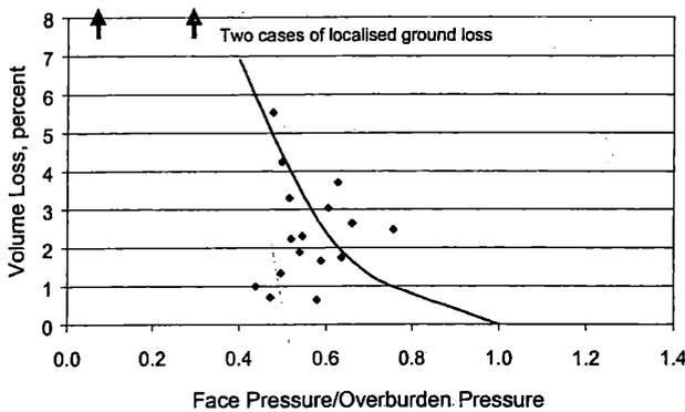
Figure 3. Relationship between face pressure and measured volume loss, EPB tunnelling through a mixed face of Kallang Formation soils and weathered rocks of the Jurong Formation
