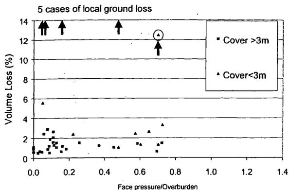
Figure 6. Relationship between face pressure and measured volume loss, EPB tunnelling through the Jurong Formation with Kallang Formation soils above the tunnel.
