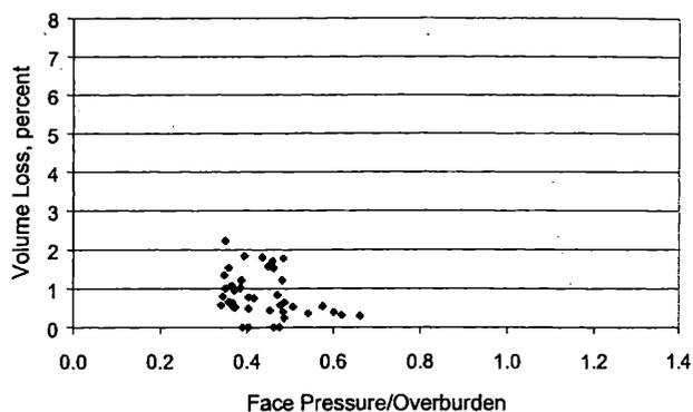
Figure 8. Relationship between face pressure and measured volume loss, EPB tunnelling through the Residual Soil of the Bukit Timah Granite.
