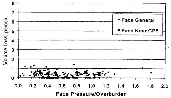
Figure 4. Relationship between face pressure and measured volume loss, EPB tunnelling through Old Alluvium
