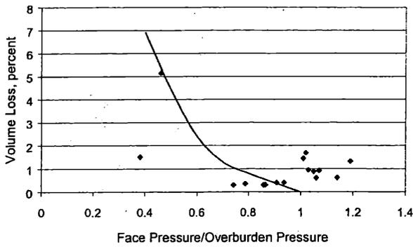
Figure 2. Relationship between face pressure and measured volume loss, EPB tunnelling through a mixed face of Kallang Formation soils and Old Alluvium
