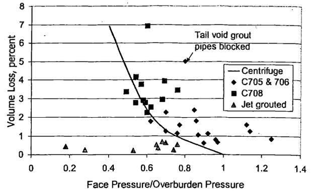
Figure 1. Relationship between face pressure and volume loss, EPB tunnelling in Kallang Formation soils.
