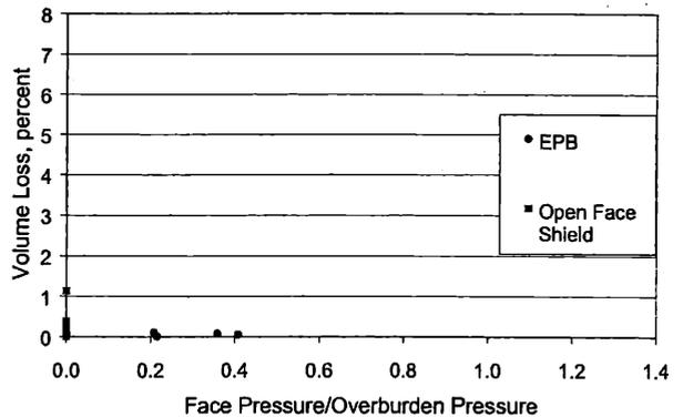
Figure 5. Relationship between face pressure and measured volume loss, EPB and open-face shield tunnelling through the Fort Canning Boulder Bed
