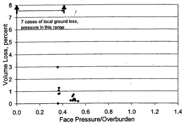
Figure 9. Relationship between face pressure and measured volume loss, EPB tunnelling through mixed weathering grades of the Bukit Timah Granite.
