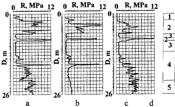
Figure 3. Results of cone penetration test (CPT):
