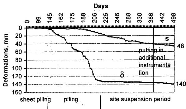
Figure 4. Plots of settlement of the residential building and displacement  $\delta$  of the sheet piles against time.
