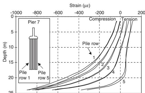
Figure 7. Strain distributions in pile group at Pier 7.
