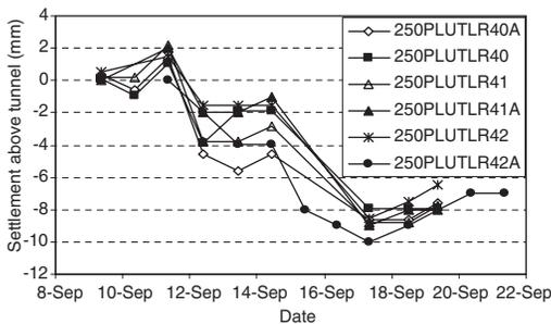
Figure 4. Settlement above upline TBM at Ripple Road.
