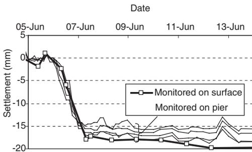
Figure 2. Settlement at Renwick Road Bridge during passage of downline TBM.
