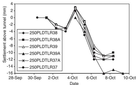
Figure 5. Settlement above downline at Ripple Road.
