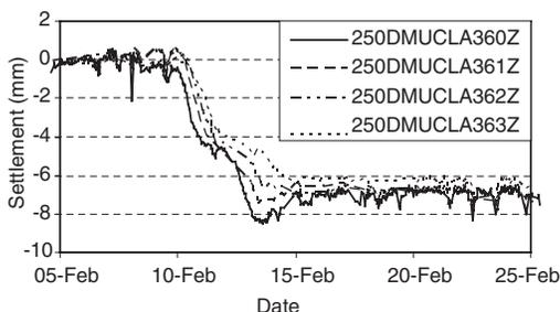
Figure 8. Surface settlements above the upline tunnel shoulder at the A406 viaduct.
