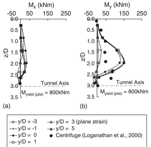
Figure 7. Tunnelling induced bending moments along the pile at various stages of excavation (a) about the x-axis and (b) about the y-axis.
