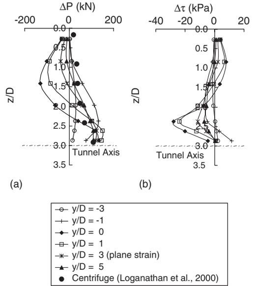
Figure 6. Changes of (a) axial force; (b) side shear stress along the pile at various stages of excavation.
