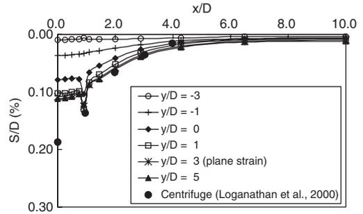
Figure 4. Transverse surface settlements induced at the monitoring section during tunnel advancement.
