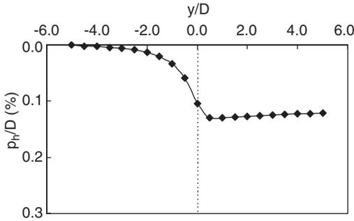
Figure 5. Pile head displacement due to tunnel excavation.
