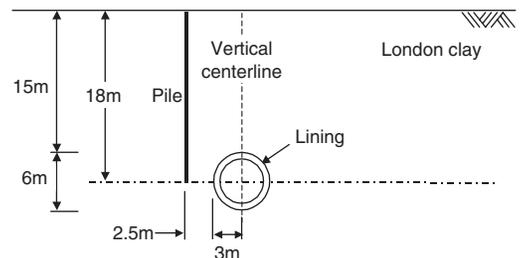
Figure 1. Ground conditions and tunnel geometry.
