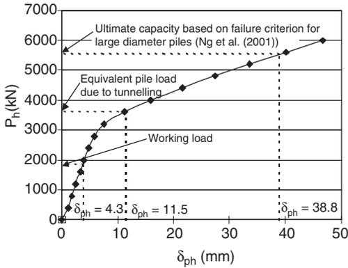
Figure 3. Pile head load vs pile head displacement.
