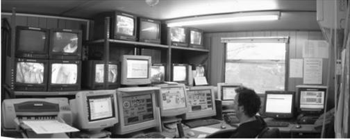
Figure 1. EPBM Control Room at Stratford. Screens show tunnel survey, TBM operation, conveyors, metro tunnel real-time monitoring, CCTV of the TBM, and environmental monitoring of the CTRL tunnel. There is also a view of the muck pile through the window that proved invaluable.
