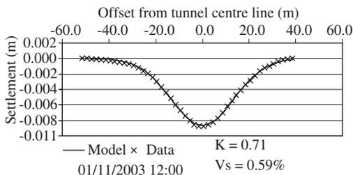
Figure 6. The result of back analysis of settlement for G.N & C southbound using Excel solver. The curves demonstrate the close agreement between the data and the model.
