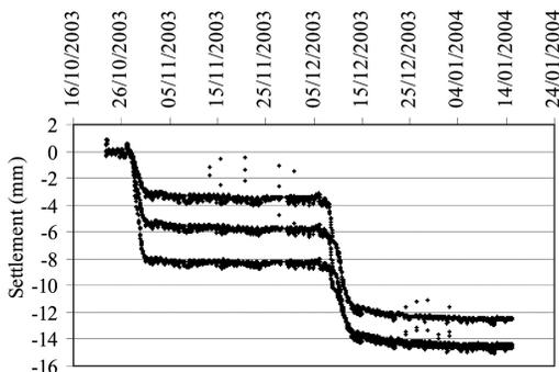
Figure 4. Settlement Time-history of GN & C northbound tunnel due to excavation of CTRL tunnels. Two events are apparent reflecting the separate passage of the two TBM's.
