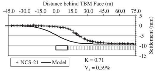
Figure 2. Settlement of GN & C southbound tunnel due to excavation of CTRL up tunnel normalized to show the development relative to CTRL TBM advance. The solid line shows the assessment. This plot confirms that the settlement in front of an EPB is small with the majority of movement occurring behind the tailskin.
