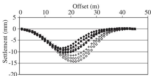
Figure 5. Transverse settlement development for GN & C northbound tunnel showing the effect of excavation for the CTRL down tunnel. The profiles show how the centre of the combined trough migrated laterally with the passage of the second TBM.
