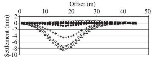
Figure 3. Transverse settlement of GN & C northbound tunnel due to excavation of CTRL up tunnel. The profiles represent 12 hour increments during the passage of the TBM.
