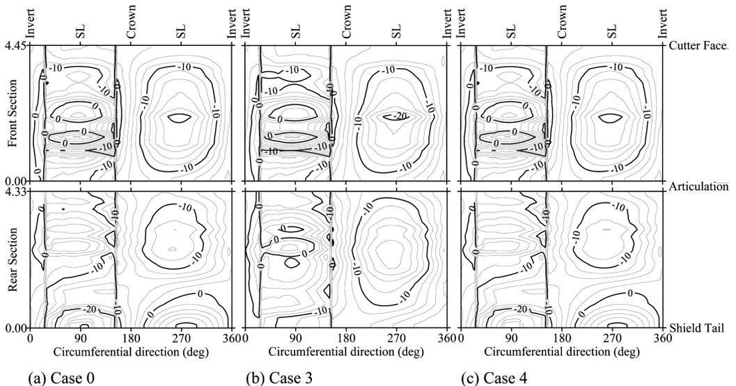
Figure 7. Gap between shield and initial excavated surface.
