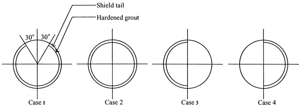
Figure 5. Cases analysed for hardened grout considerations.
