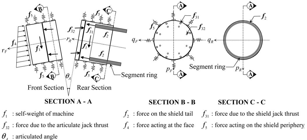
Figure 2. Model of loads acting on articulated shield.
