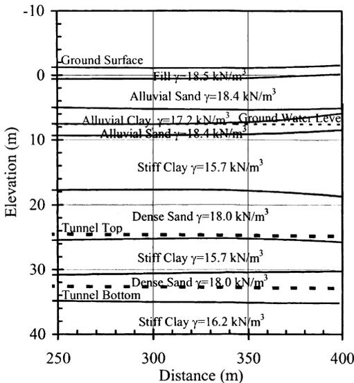
Figure 3. Geological profile at test site location.
