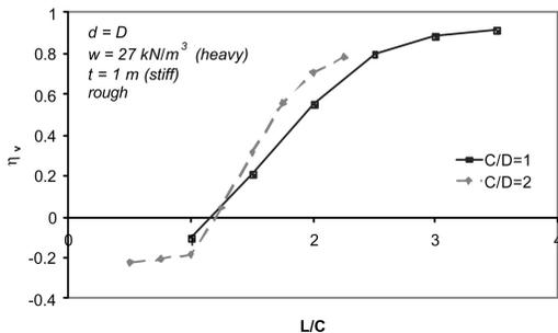
Figure 14. Efficiency of heavy, stiff and rough walls with L/C.
