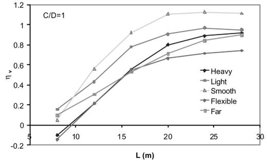
Figure 13. Efficiency of different kind of walls with length.
