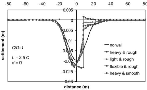
Figure 7. Comparison of settlement profiles: different kind of walls of the same length.
