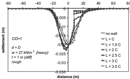
Figure 3. Comparison of settlement profiles: rough, stiff and heavy walls of various lengths.
