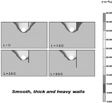
Figure 11. Displacement filled contours at  $V' = 1\%$  – smooth walls.
