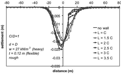
Figure 6. Comparison of settlement profiles: rough, flexible and heavy walls of various lengths.
