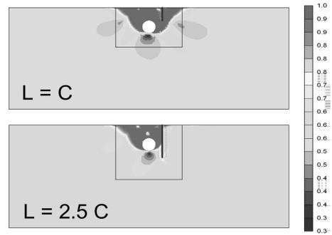
Figure 9. Relative shear stress filled contours at collapse.
