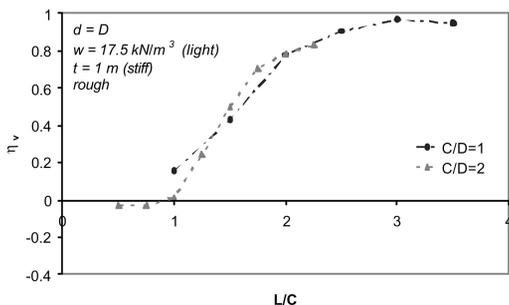
Figure 15. Efficiency of light, stiff and rough walls with L/C.
