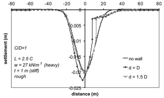
Figure 8. Comparison of settlement profiles: same wall at two different location ( $D$  and  $1.5 D$  away from the tunnel axis).
