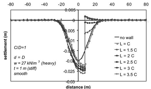
Figure 5. Comparison of settlement profiles: smooth, stiff and heavy walls of various lengths.
