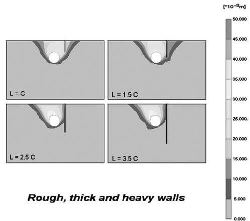
Figure 10. Displacement filled contours at  $V' = 1\%$  – rough walls.
