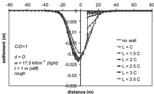
Figure 4. Comparison of settlement profiles: rough, stiff and light walls of various lengths.
