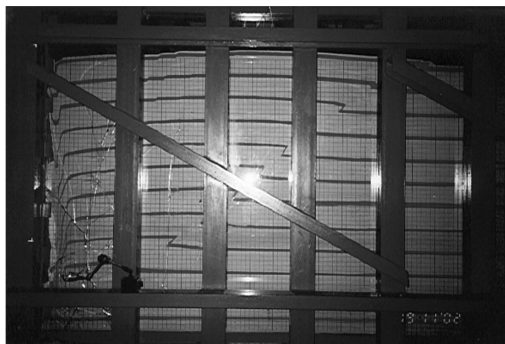
Figure 2. The state of the mass and the first glass plate near the moved wall (left) after the toe movement of 134.8 mm before the final movement of 159 mm on 18th Nov. 2002. The destroyed glass plate resisted the stress state with the pressure of 150 kPa.
