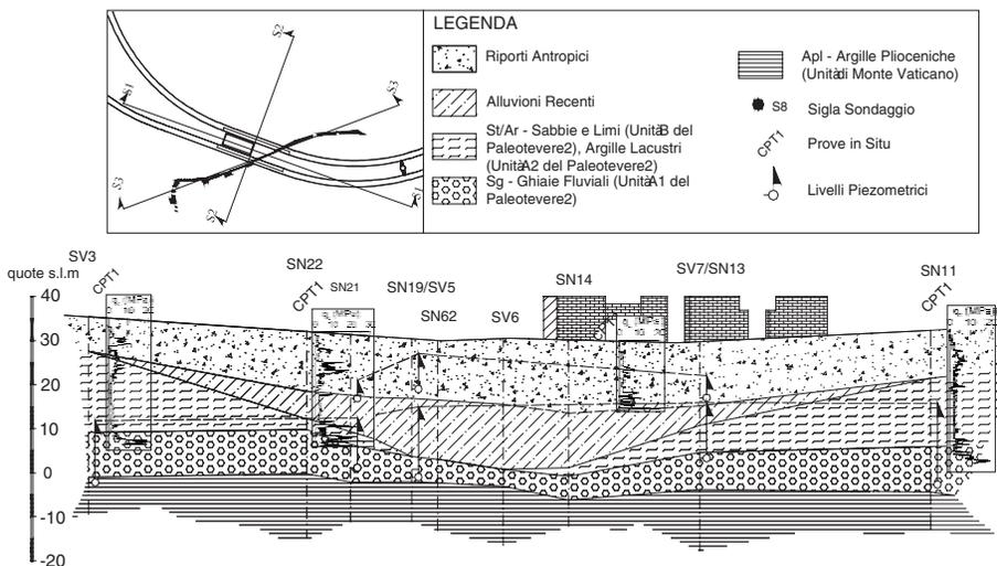
Figure 4. Geotechnical profile parallel to the tunnel axes.
