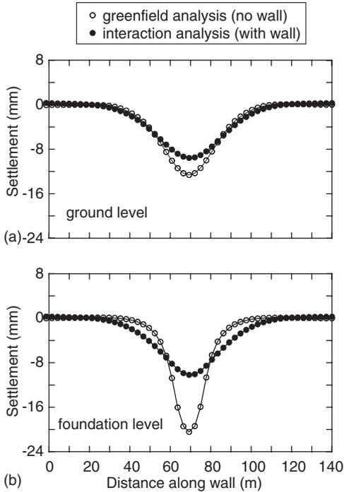
Figure 8. Vertical displacements along the wall: (a) ground level, (b) foundation level.
