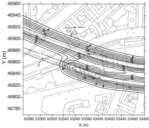
Figure 6. Surface settlement contours (mm,  $V_S = 1.0\%$ ).
