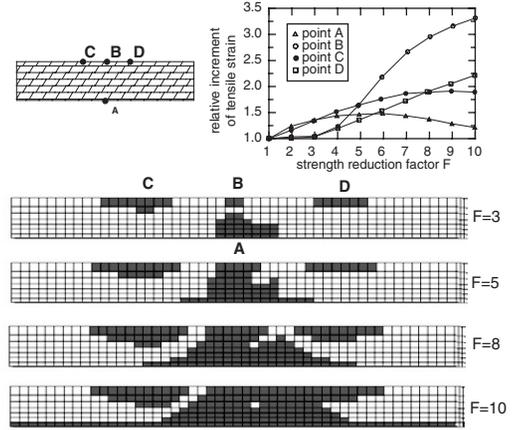
Figure 11. Effects of a strength reduction on the computed maximum tensile strains.
