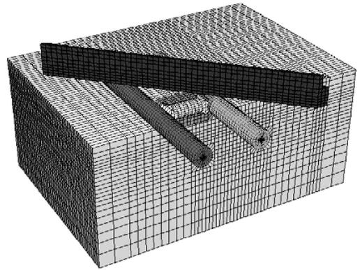
Figure 7. Three-dimensional mesh adopted for the analyses.
