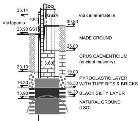
Figure 5. Schematic section through the Aurelian Wall at Largo Amba Aradam.
