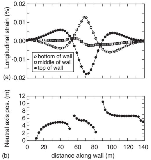
Figure 9. (a) Computed maximum tensile strain in the mid plane of the Wall and (b) neutral axis position.
