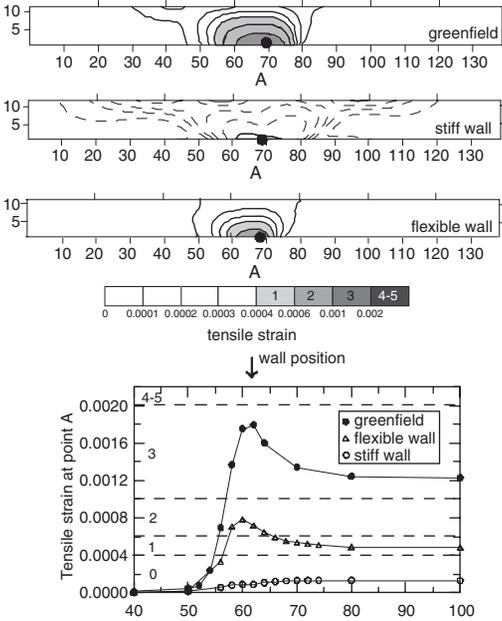
Figure 10. Contours of maximum tensile strain and corresponding levels of damage.
