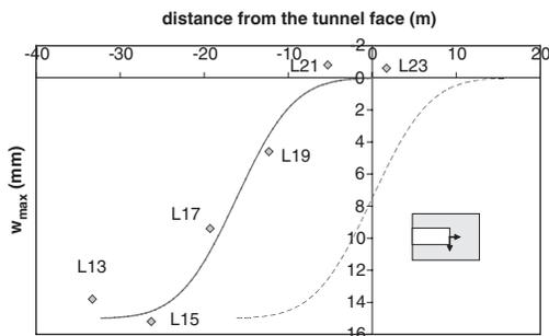
Figure 9. Longitudinal profile of settlement vs distance from face.
