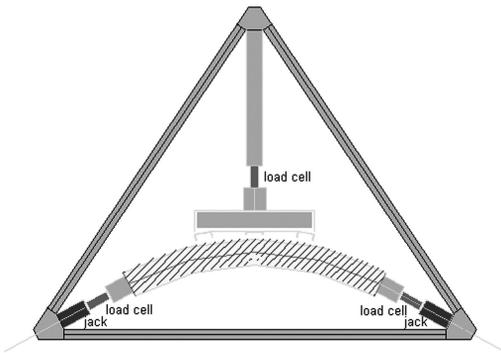
Figure 4. Schematic plan view of the experimental layout.
