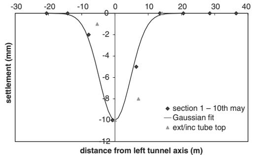
Figure 6. Measured settlement in section 1.
