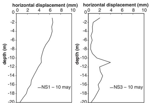
Figure 7. Horizontal displacements measured in section 1.
