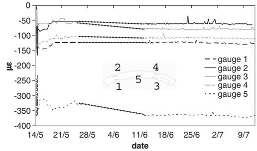
Figure 12. Measured strains in segment D4 after installation.
