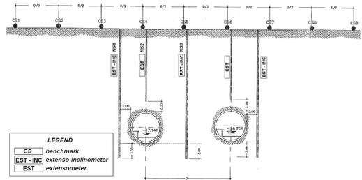
Figure 1. Typical layout of an instrumented cross section.
