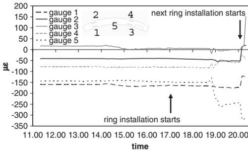
Figure 11. Measured strains in segment D4 during installation inside the shield tail.
