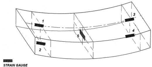
Figure 2. Location of the strain gauges in the instrumented segments.
