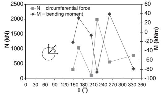
Figure 13. Circumferential force and bending moment in the ring.
