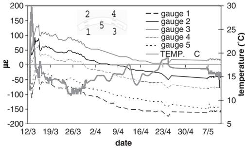
Figure 10. Measured strains in segment D4 during the curing stage.
