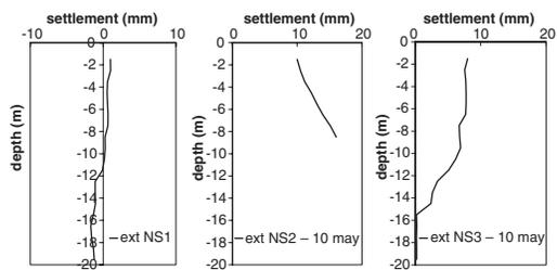
Figure 8. Deep settlement measured in section 1.
