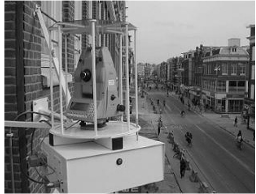
Figure 3. Robotic total station.
