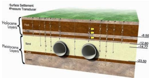
Figure 5. Sophia Rail Tunnel, soil stratification and location of extensometers at the measurement location (picture Arne Bezuijen).
