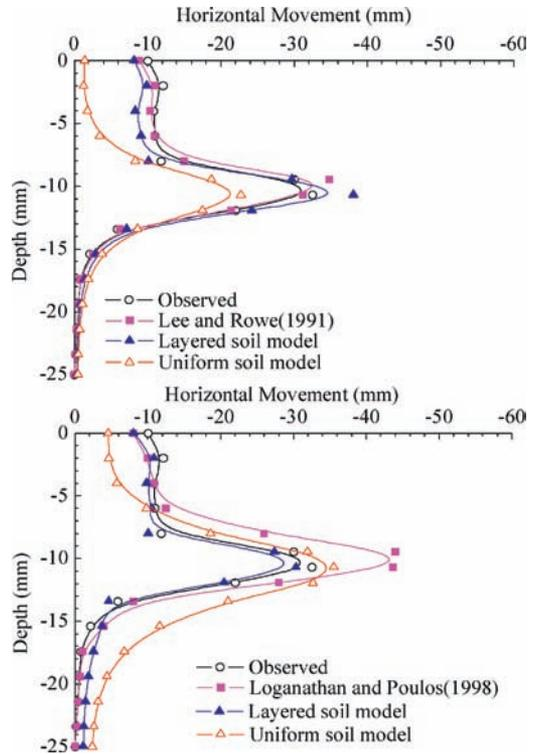
Figure 9. Lateral displacement 15 m behind the tunnel face.
