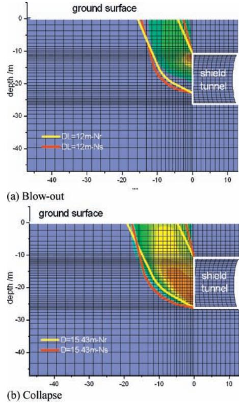
Figure 3. Comparison of failure mechanisms of Case 2 (velocity contour for FLAC<sup>3D</sup> analysis).
