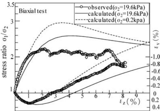
Figure 1. Stress-strain-dilatancy relation.
