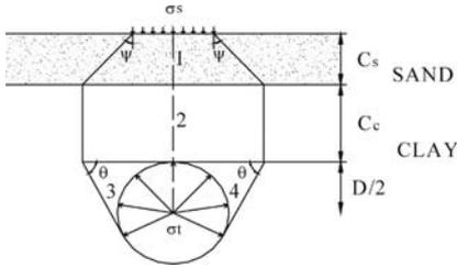
Figure 5. Mechanism of failure for layered ground.
