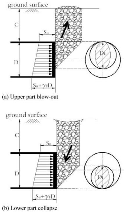
Figure 2. Two kinds of partial failure mechanisms.
