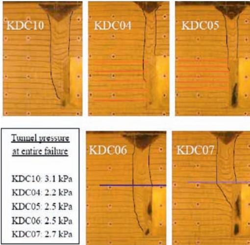
Figure 6. Tunnel failure patterns on the longitudinal section.
