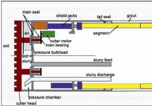
Figure 1. Sketch of a slurry shield TBM.
