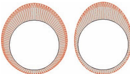
Figure 5. Deformation pattern around tunnel due to a pressure increase of 50 kPa starting at a pressure of 350 kPa (left), resulting in a maximum displacement of 22 mm. Right the same calculations but first a stress reduction to 320 kPa was applied, resulting in a max deformation of 25 mm.
