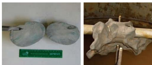
Figure 1. Results from Cambridge University (left) and GeoDelft that show more a spherical shape than fractures.
