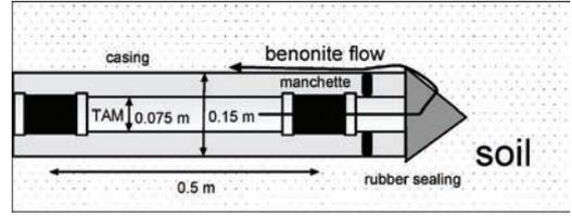
Figure 6. Sketch of casing and TAM during installation.
