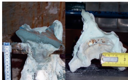
Figure 9. Dehydrated layer around the boundary of hardened grout for (a) Test 6 (left) and (b) Test 7 (right).
