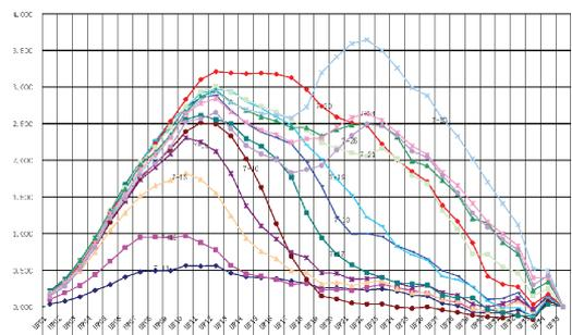
Figure 9. The Line 2 up line tunnel settlement/uplift data during the second tunneling cross process.
