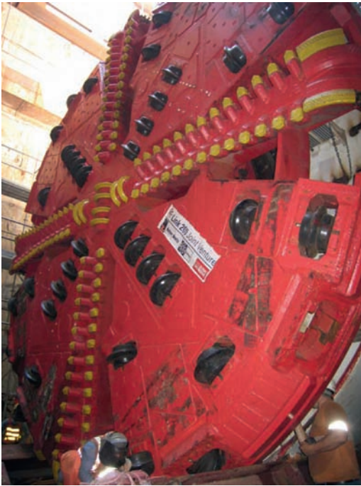
Figure 2. Slurry-type tunnel boring machine.
