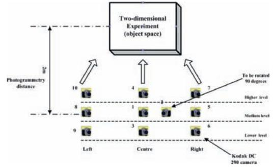
Figure 6. Typical digital camera positions for capturing 10 images.
