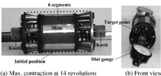
Figure 2. Diameter reduction system of model tunnel.
