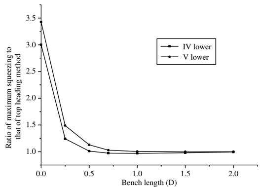
Figure 6. Relationship between bench length and maximum squeezing displacement.
