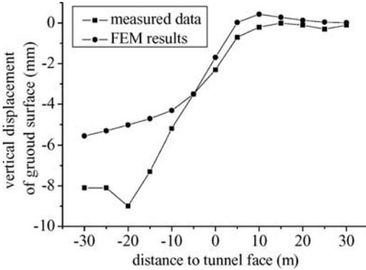
Figure 2. Displacements of ground surface along pipe axis.
