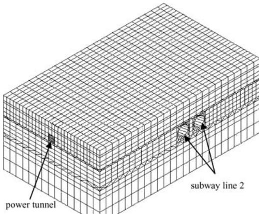
Figure 11. Mesh of power tunnel and subway line 2.
