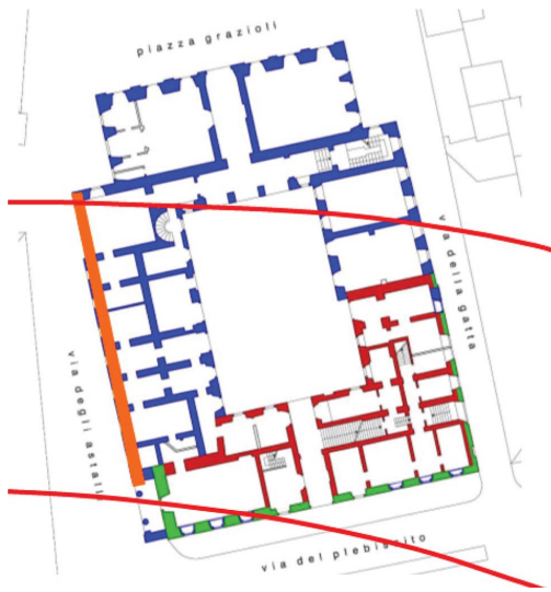
Figure 13. Plan view of Palazzo Grazioli, showing the relative position of the building and the tunnels axes.
