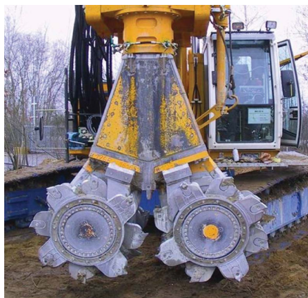
Figure 8. Mixing wheels and housing for hydraulic gear drives of a CSM unit (from Gerressen and Vohs).
