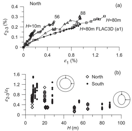
Figure 10. (a) Mean deformation  $\varepsilon_{2-3}$  of the two oblique control lengths against the horizontal deformation  $\varepsilon_1$  from several monitoring sections (open symbols) and from FLAC3D analyses (full symbols) at different overburden  $H$ . (b) Ratio between measured deformations of oblique and horizontal control lengths related to overburden  $H$ .
