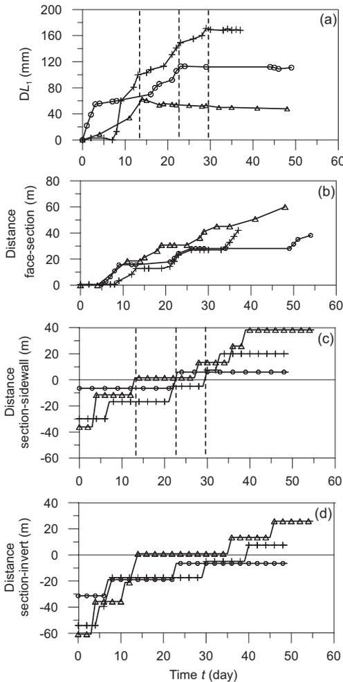
Figure 7. Time histories of: a) the measured convergence of the horizontal closure  $L_1$ ; b), c) and d) the progression of the face, sidewall and invert concrete, respectively, with reference to the control section position. The vertical lines refers to the time of casting of the sidewall.
