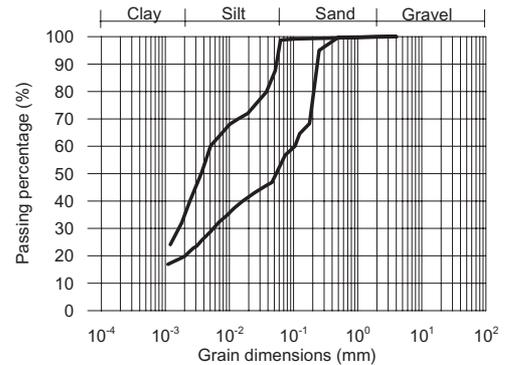
Figure 2. Two limit grain-size distributions of soil samples collected at the tunnel face.
