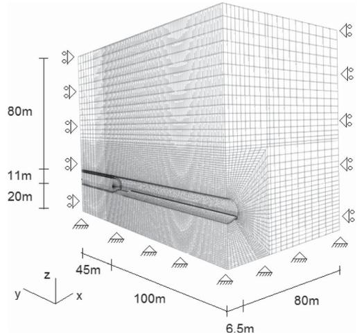
Figure 11. Calculation mesh including boundary constraints.
