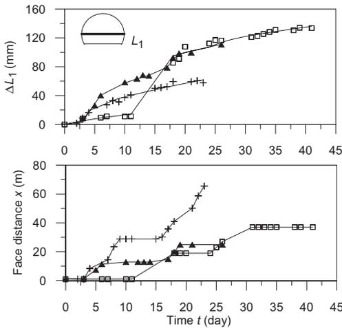
Figure 5. Examples of curve fitting (continuous line) of convergence measurements  $\Delta L_1$  (symbols) with time (on the top) at three monitoring sections. At the bottom the distance of the monitoring section from tunnel face versus time is shown.
