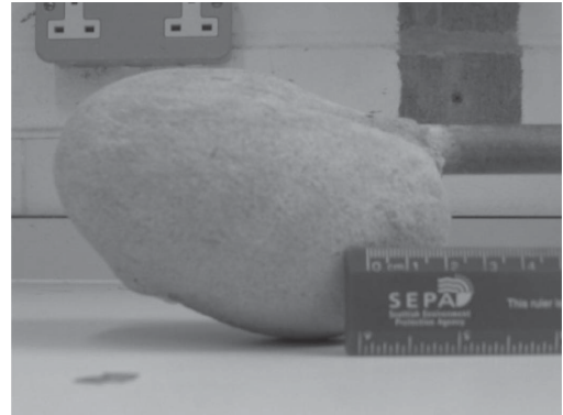
Figure 8. Hardened grout for w/c = 0.5 and b.c. = 4%.
