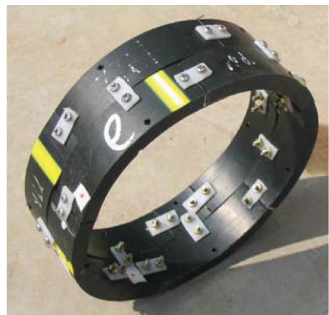
Figure 3. The assembly of the tunnel segments.
