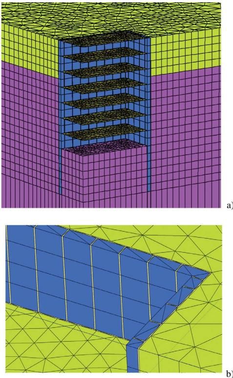
Figure 3. Details of the 3D mesh: a) walls and slabs; b) panel interfaces.
