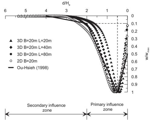
Figure 9. Normalized ground settlement profiles ( $H_e = 28$  m).
