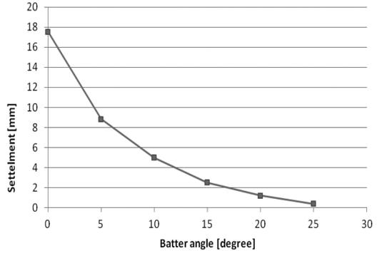
Figure 6. Effect of batter angle variations on settlements.
