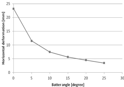
Figure 5. Effect of batter angle variations on horizontal deformations.
