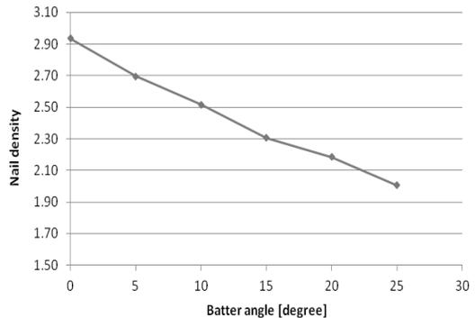
Figure 7. Effect of batter angle variations on Nail density.
