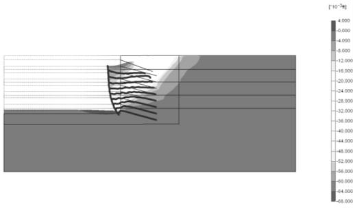
Figure 3. Horizontal displacement of the Polyclinic wall model.
