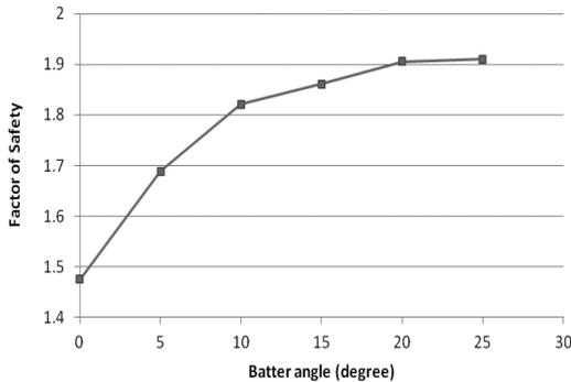
Figure 4. Effect of batter angle variations on factor of safety.
