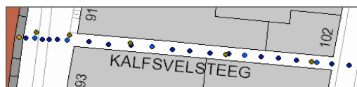
Figure 6. Measurement array at RKN Station with surface measurements (blue dots), inclinometers and extensometers (brown dots).
