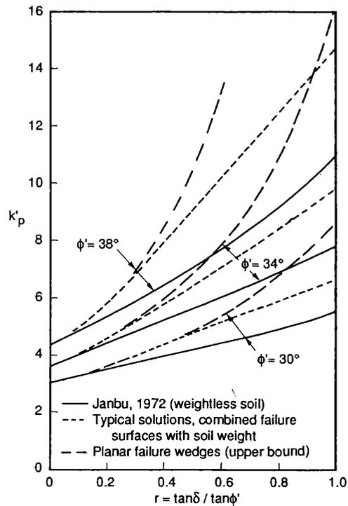
Figure 3. Effective passive earth pressure coefficients (for  $|r| \geq 0$ ).
