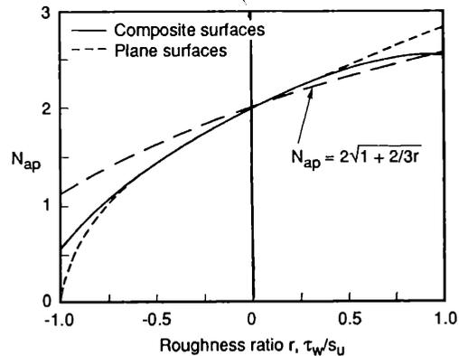
Figure 2. Total stress active and passive earth pressure coefficients (Janbu, 1972).
