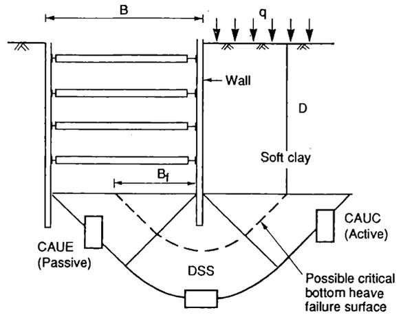
Figure 1. Illustration of base heave failure mechanism.
