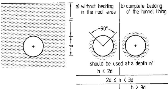
Figure 11 Assumptions for soil-lining-interaction, AK 10 (1980)
