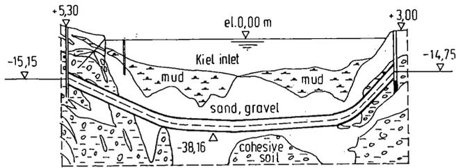
Figure 7 Use of a compressed air shield under the Kiel inlet (Kieler Förde). Geological cross section, BARG, THIEMANN (1990)
