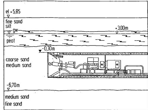
Figure 5 Tube heading of a sewer in Hamburg, STADT HAMBURG (1988) (slightly changed)
