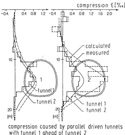
Figure 13 Metro Munich, staggered parallel heading of two tunnels, measured vs. computed subsoil compression, KOVARI, AMSTAD (1987)
