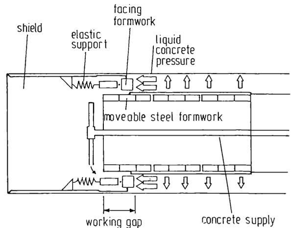
Figure 10 Metro Essen, earth pressure shield with extru-concrete support, WITTKÉ (1989)
