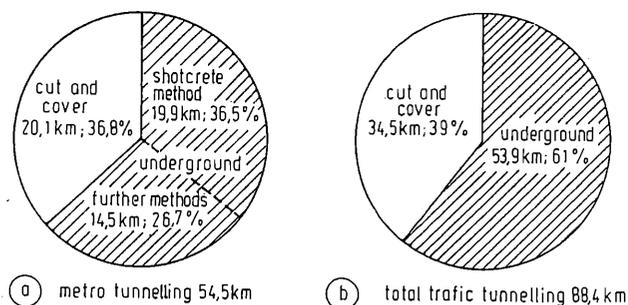
Figure 1 Shares of construction methods in German traffic tunneling, end of 1990, HAACK (1991)
