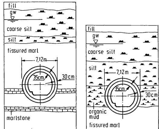
Figure 6 Metro Essen, use of an earth pressure shield in varying geological conditions, HOCHTIEF (1988)
