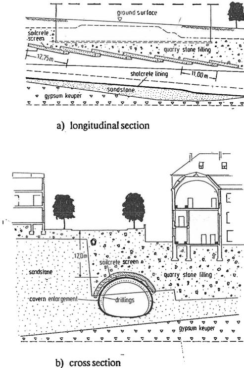
Figure 3 Expo tunnel, Stuttgart, tunneling with an advancing soilcrete screen, BEICHE et al. (1992)
