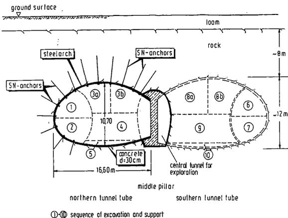
Figure 4 Road tunnel, Wuppertal, driving of a large cross section in partial headings, MODEMANN, WITTKÉ (1987)
