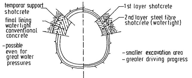
Figure 9 Shotcrete support, comparison of single and double lining, MAIDL, KOENNING (1989)
