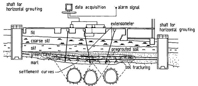
Figure 14 Metro Essen, undercrossing of an industrial building, measuring and grouting scheme, STADT ESSEN (1987)
