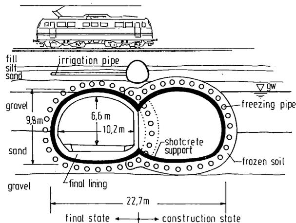
Figure 2 Fahrlach tunnel, Mannheim, tunneling with frozen soil support, DUSCH, MAYER (1989)
