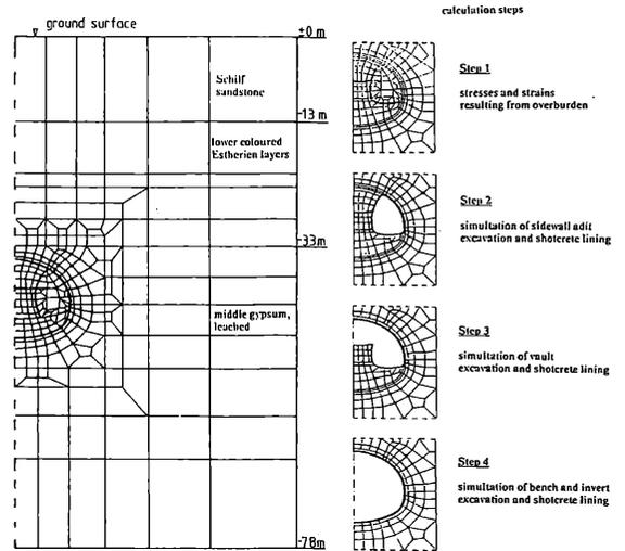
Figure 12 Road tunnel Stuttgart-Heslach II, FE mesh, WITTKÉ (1987)
