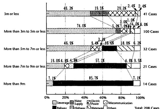
Figure 5. Tunnel usage classified by outer diameter of RC segment
