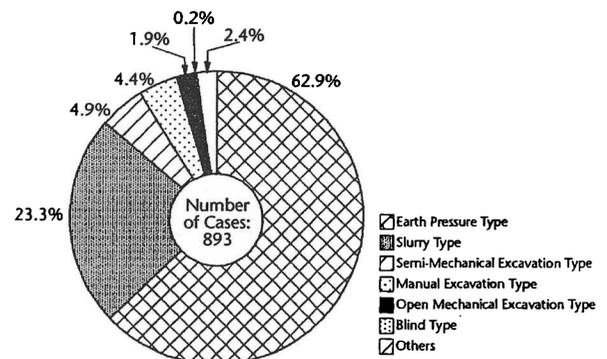
Figure 1. Percentage of application of each shield tunneling methods (1987 to 1992)
