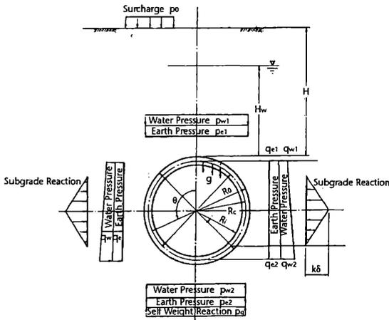
Figure 6. Example of design earth and water pressures acting on segment ring
