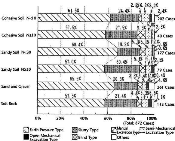
Figure 2. Relationship between shield tunneling methods and typical soil conditions at cutting face
