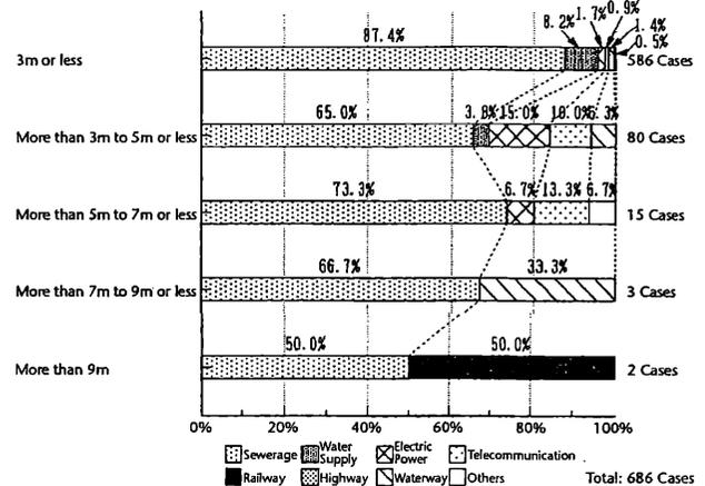
Figure 4. Tunnel usage classified by outer diameter of steel segment
