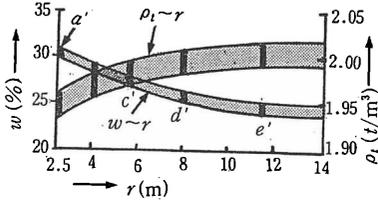
Fig.8 Increase in water content and decrease in wet density in a plastic zone
