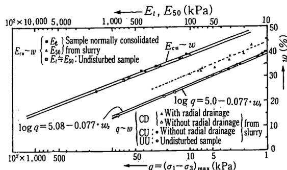
Fig.3 Relationships between compressive strength  $q$ , Young's modulus  $E_{cu}$  and water content  $w$
