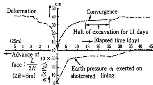
Fig.2 Increase in earth pressure and convergence in relation to the advance of tunnel face and elapsed time
