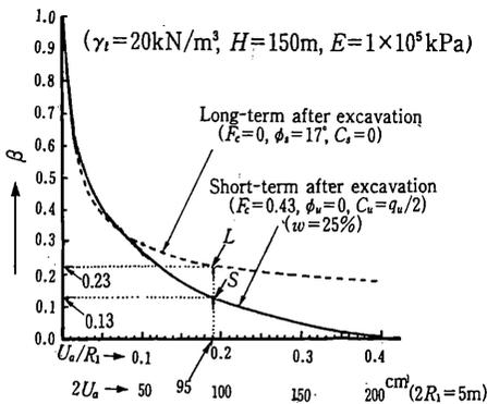
Fig. 6 Relationship between  $\beta = \sigma_i / (\gamma_t \cdot H)$  and convergence  $2U_a$ .
