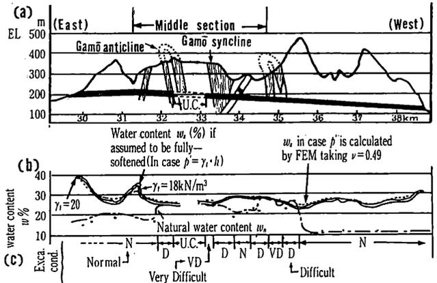
Fig.1 Profile of Nabetachiyama Tunnel
