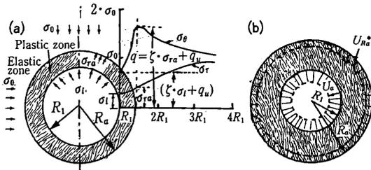
Fig. 5 Stresses around a deep circular tunnel in elastic-plastic state (a) and deformation (b)
