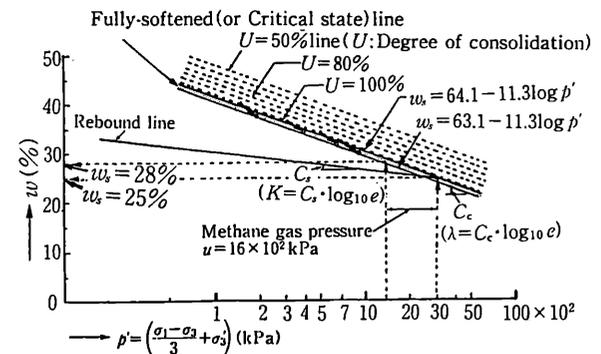
Fig.4 Relationship between average effective confining stress  $p'$  and water content  $w$
