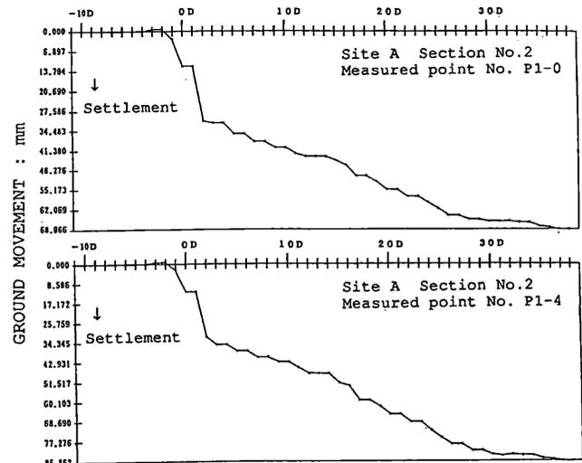
Fig.7 Ground movements of Site A, Section No.2
