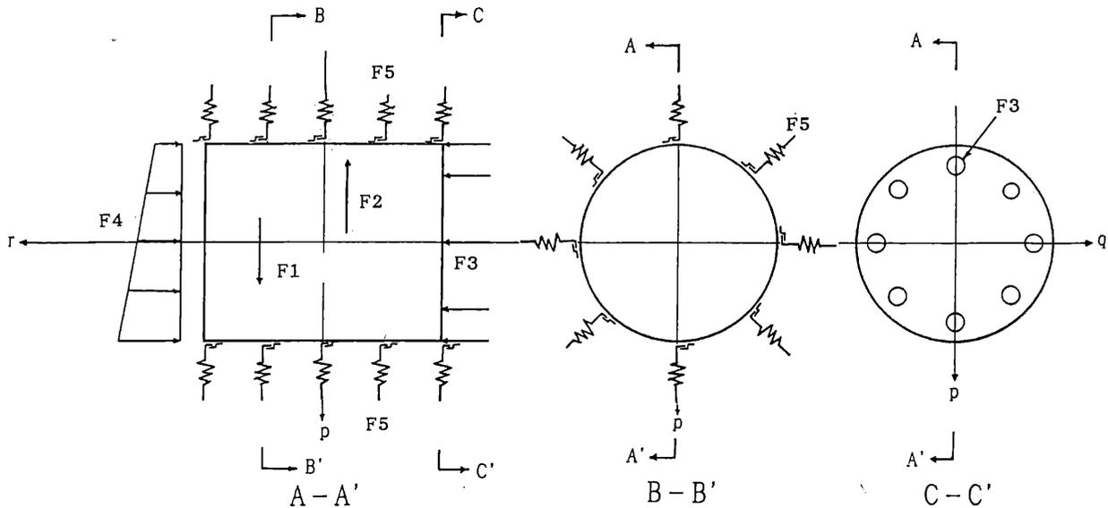
Fig. 1. Model of acting load on shield
