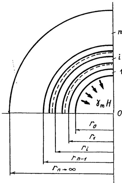
Figure 1. General design scheme for a multi-layer diaphragm wall:  $i = 1, 2, \dots, (n-1)$  is the number of the layer,  $n$  is the infinity layer, simulating soil mass.
