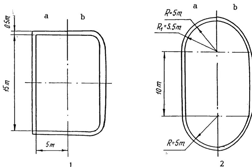
Figure 4. Rectangular (1) and oval (2) shapes in plane diaphragm walls for designing: 1 - project forms, 2 - shapes after conformal mapping.
