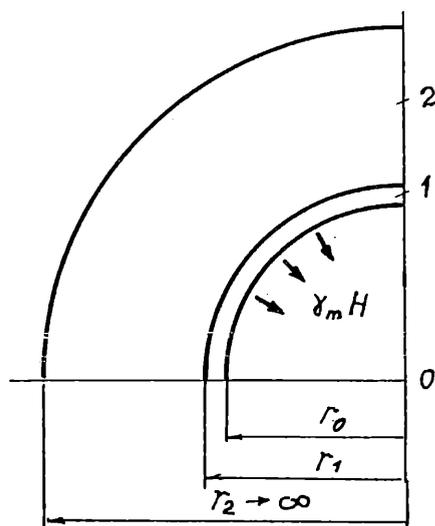
Figure 3. Design scheme of the shaft diaphragm wall.
