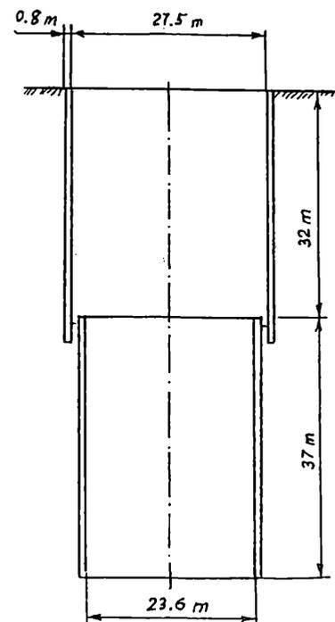
Figure 2. Scheme of the shaft.
