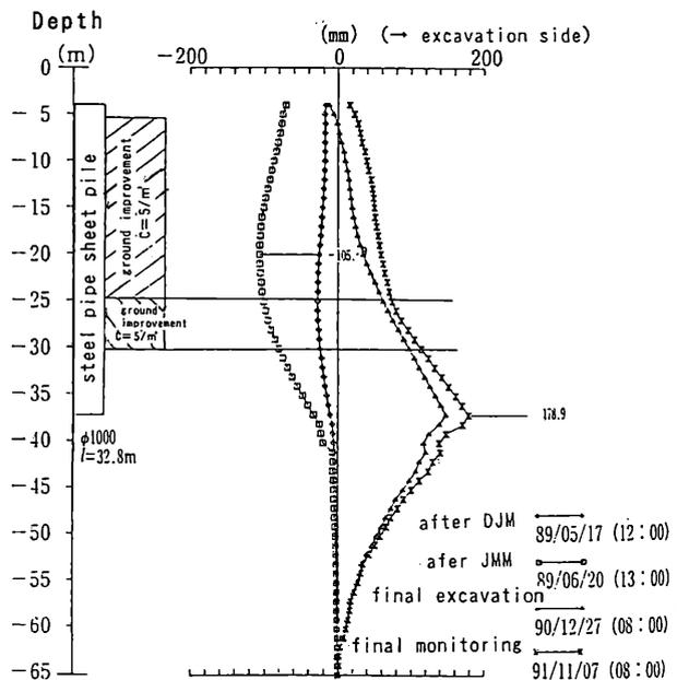
Fig-8. Deformation of the retaining wall
