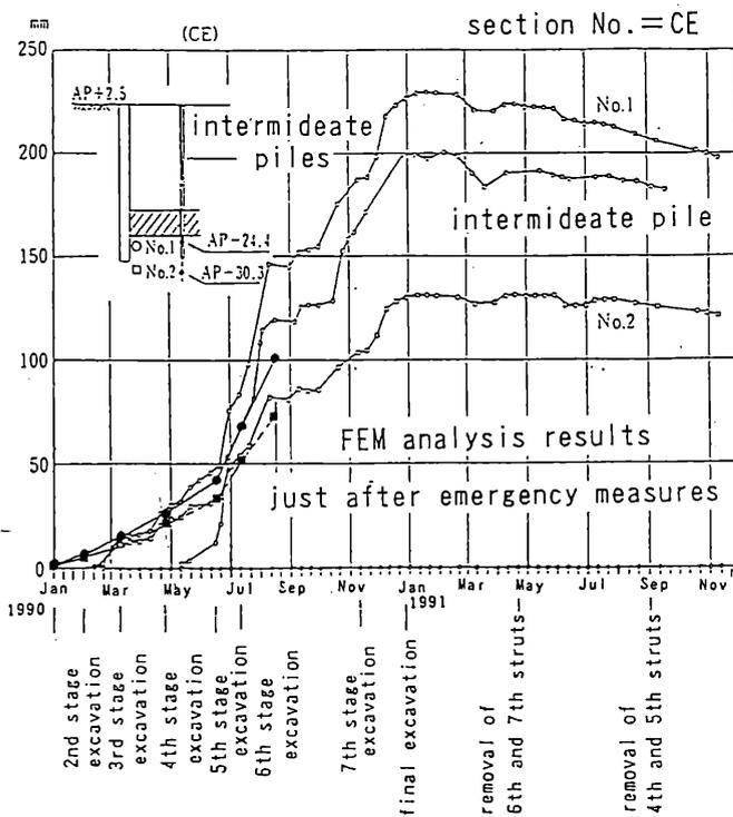
Fig-7. Ground heaving during excavation
