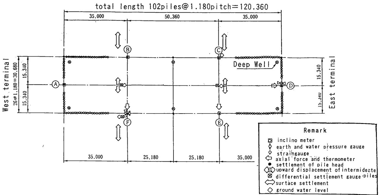
Fig-6. Layout plan for the measuring instruments
