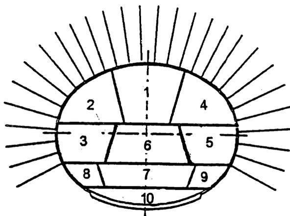
Figure 6: Typical excavation sequence of NATM underground stations. Width=16.5m, height=12.7m.
