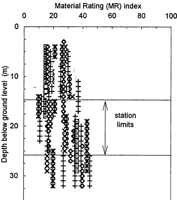
Figure 2: Distribution of the MR index with depth. Results from ten boreholes in the area of the Omonia station.
