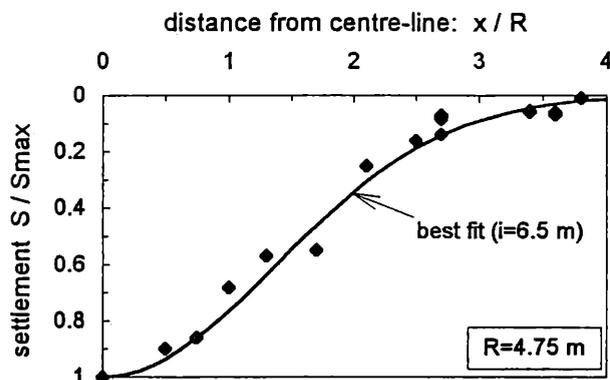
Figure 5: Normalised shape of the surface settlement trough. Line 2 TBM tunnel.
