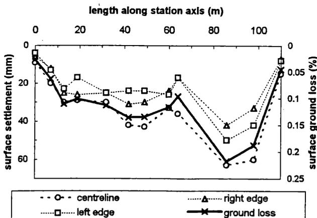
Figure 7: Surface settlement distribution and ground loss along the Omonia underground station.
