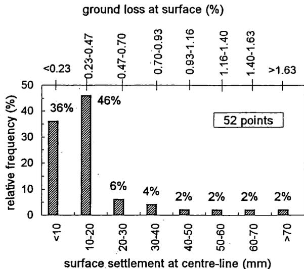
Figure 4: Frequency distribution of the measured surface settlements above the tunnel centreline and ground loss at surface level. Line 2 TBM tunnel.
