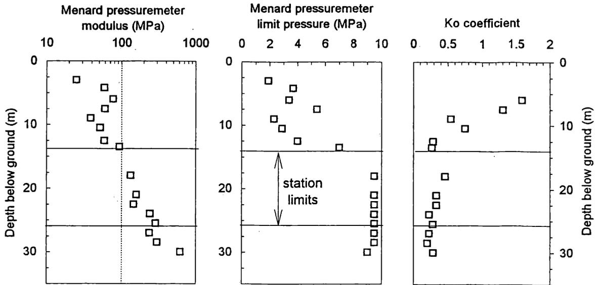
Figure 1: Menard-type pressuremeter test results from boreholes at the Omonia underground station.
