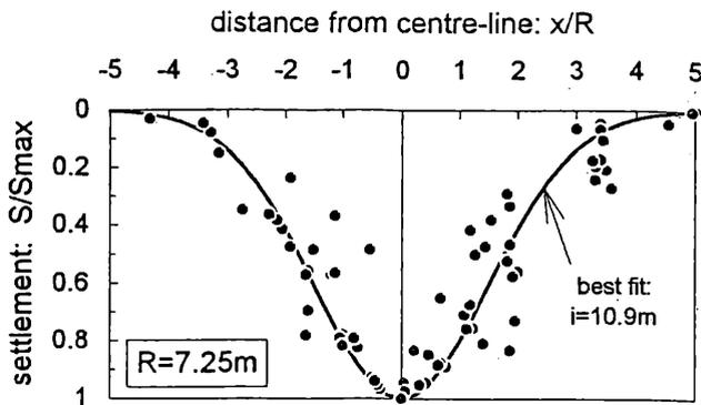
Figure 8: Normalised surface settlement trough at Omonia underground station.
