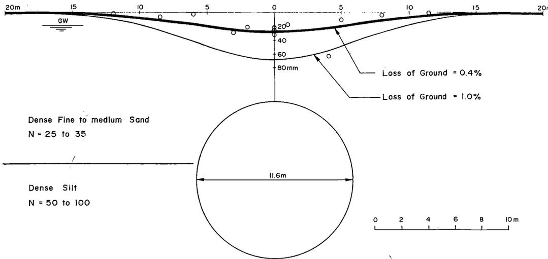
Fig. 6 Observed Settlements induced by tunnelling below State Road T1.
