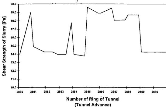
Fig. 4 Shear strength of slurry near cavern 28
