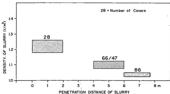
Fig. 5 Slurry Penetration as a function of density
