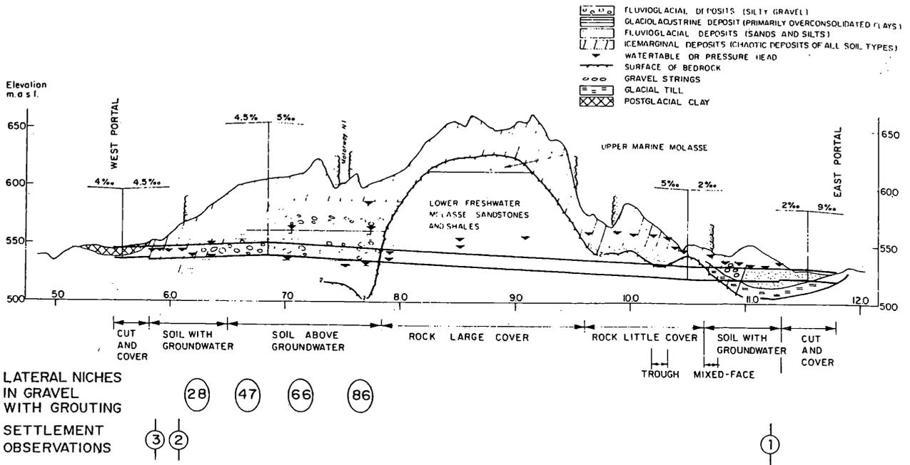
Fig. 1 Geologic Section along Grauholz tunnel with observation points of slurry penetration and settlements
