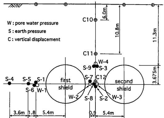
Fig.5 Location of instruments
