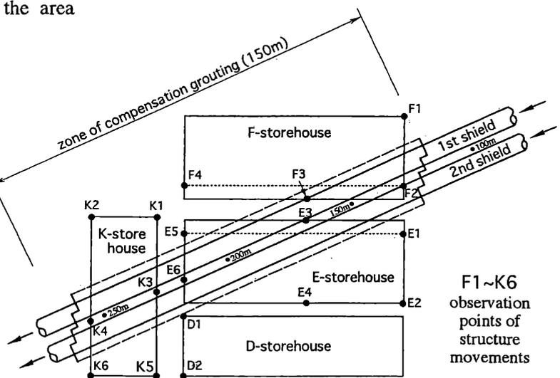
Fig.1 Plan location of two parallel shield tunnels and existing storehouses
