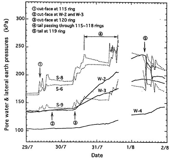
Fig.8 Changes of pore water and earth pressures during the passage of the first shield
