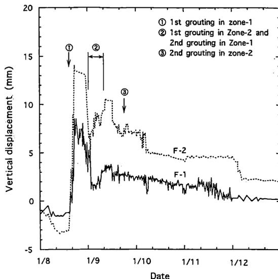
**Fig.10** Movement of F-storehouse during tunnelling
