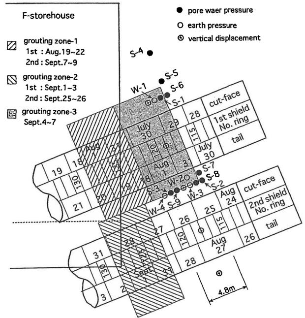
Fig.4 Layout of instruments and advancing schedule of shields
