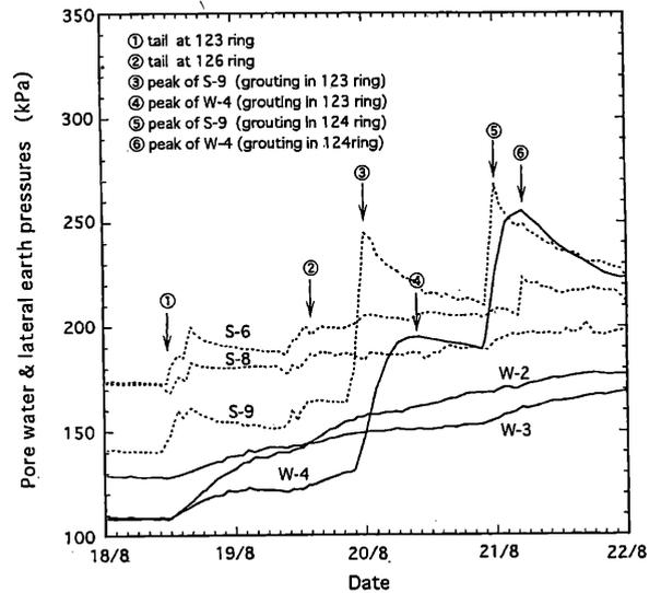
Fig.9 Changes of pore water and earth pressures during compensation grouting (Zone-1)
