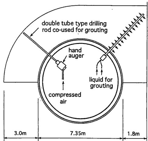
Fig.3 Details of compensation grouting
