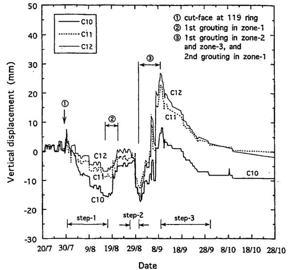
**Fig.6** Ground movement observed during tunnelling
