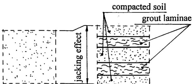
a) natural soil      b) laminated soil after grouting
