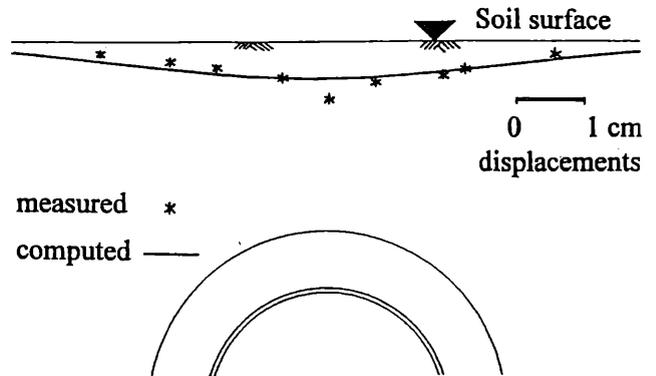
Fig. 6. Measured vs. computed surface displacements
