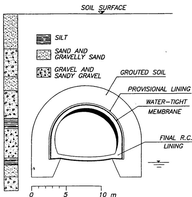
Fig. 1. Typical tunnel section and soil profile
