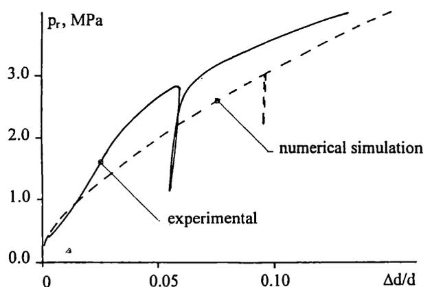
Fig. 3. Pressuremeter test results and numerical simulation.
