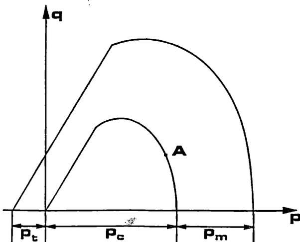
Fig. 4. Failure envelope for 'X-Lamber' model
