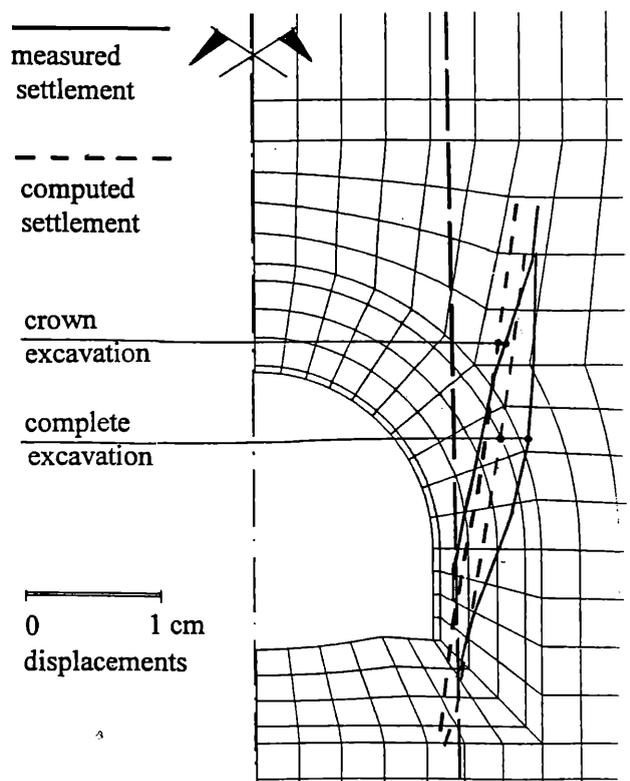
Fig. 7. Vertical displacements within soil mass. Measured vs. computed.
