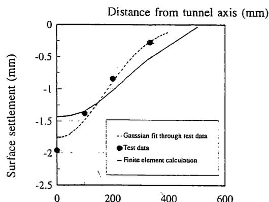
Figure 6. Measured and calculated settlement trough, expressed in model quantities.
