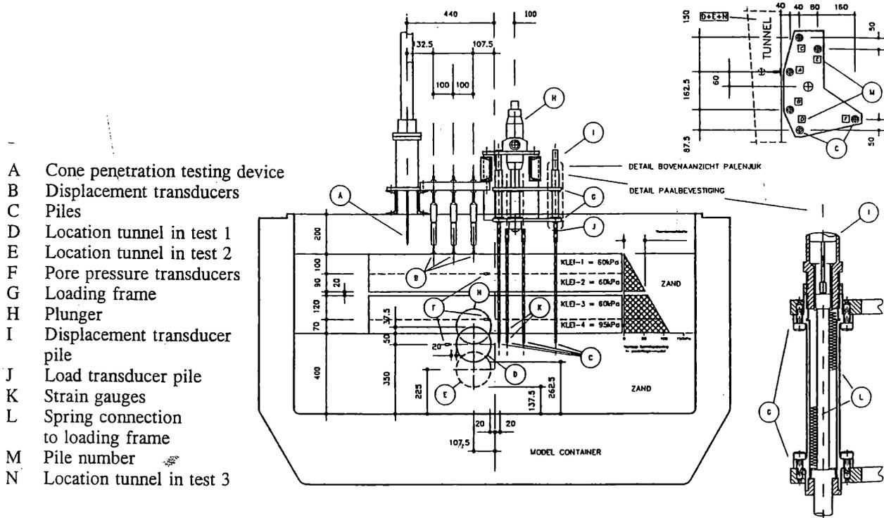
Figure 1. Section through the centrifuge model. Quantities are expressed in model values (mm).
