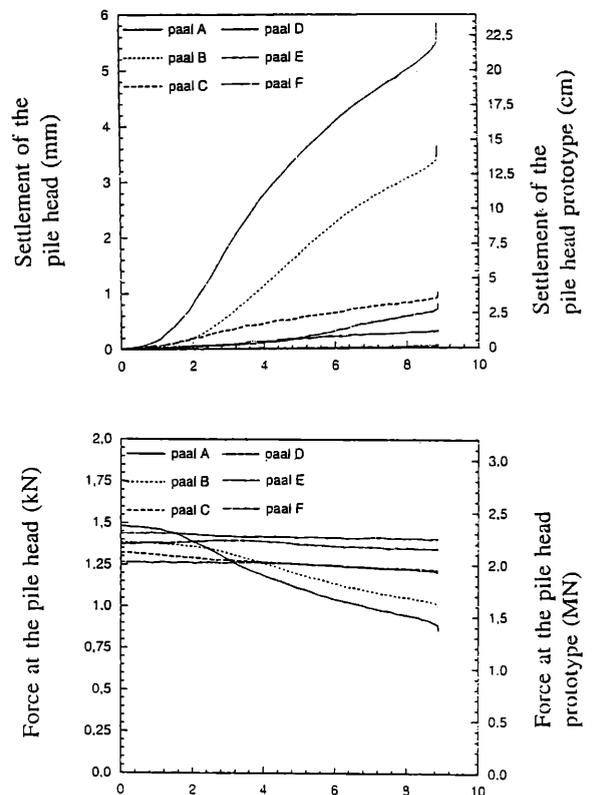
Figure 5. Results of centrifuge test in case of test 3. The piles are loaded up to a level equal to 70 % of the during the penetration phase recorded ultimate bearing capacity.
