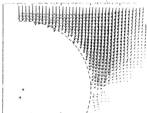
Figure 3. Image showing total displacement vectors in the clay around the tunnel.
