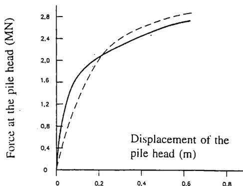
Figure 7. Pile installation. Experimental data compared to calculation result (quantities are converted to prototype values).
