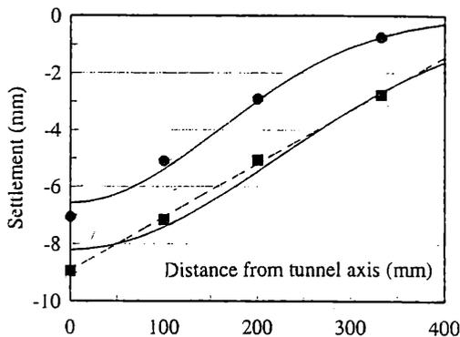
Figure 4. Settlement trough at surface level in case of test 3 (just after imposing the total volume loss of approximately 10 % and after full consolidation). The values are expressed in model quantities.
