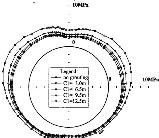
Figure 6. Hoop stresses in tunnel lining - Influence of grouting array level ( $C_1$ )
