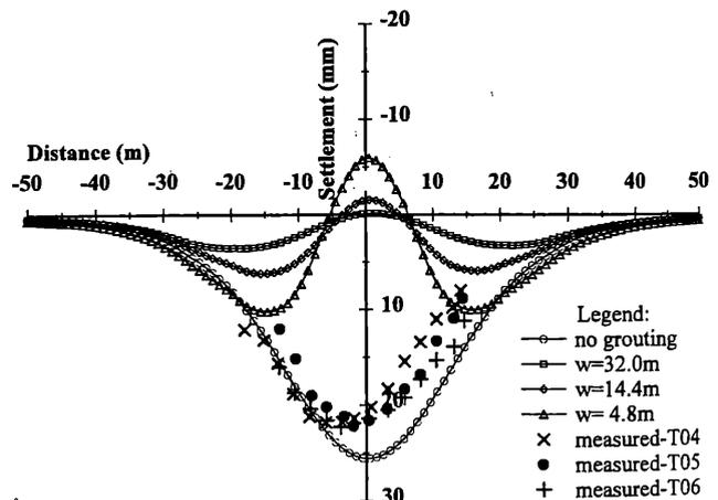
Figure 5. Surface settlement before and after compensation grouting - Influence of grouting array extent ( $w$ )
