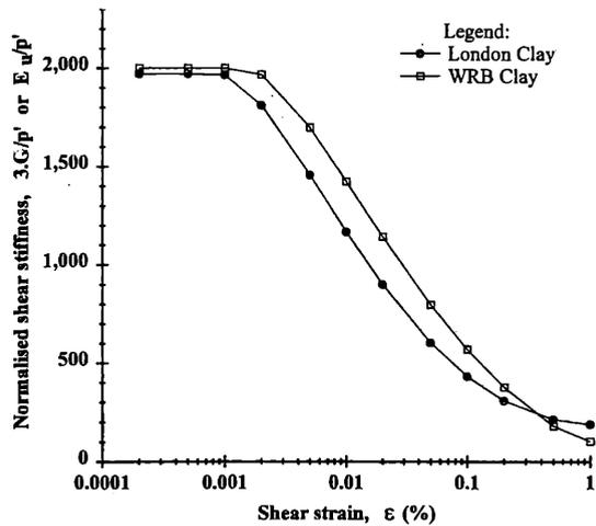
Figure 3. Adopted non-linear elastic small strain stiffness for London Clay and WRB Clay
