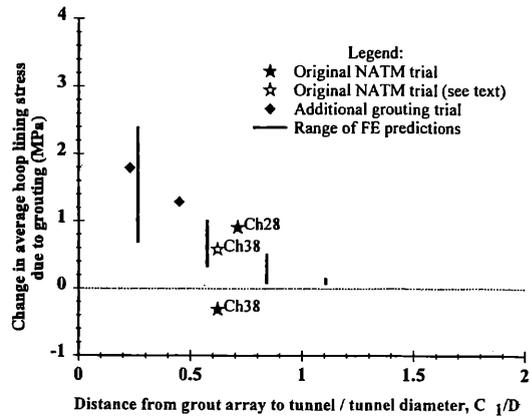
Figure 7. Changes in measured and predicted average hoop lining stresses due to compensation grouting for different values of  $C_1/D$
