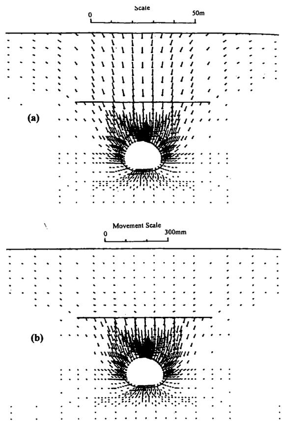
Figure 4. Accumulated displacement vectors after (a) tunnel excavation (without compensation grouting) and (b) compensation grouting
