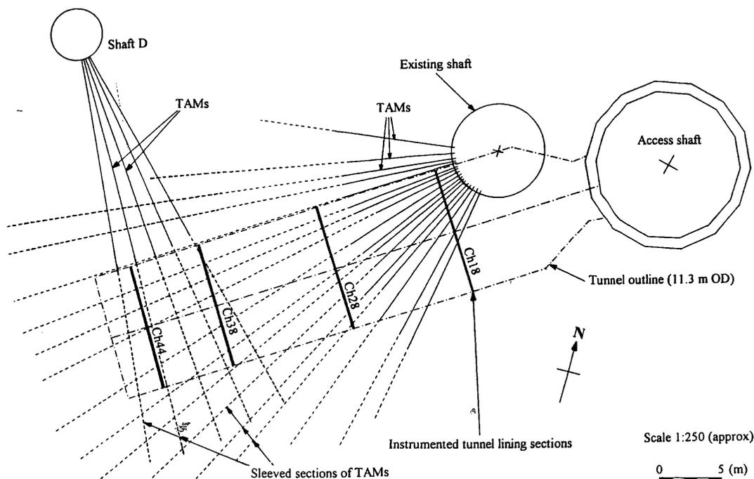
Figure 1. Plan layout of compensation grouting trials at Redcross Way
