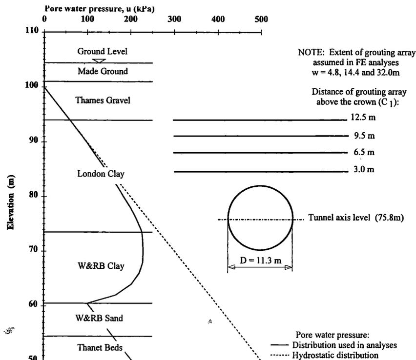
Figure 2. Soil and pore water pressure profiles, and grouting levels assumed
